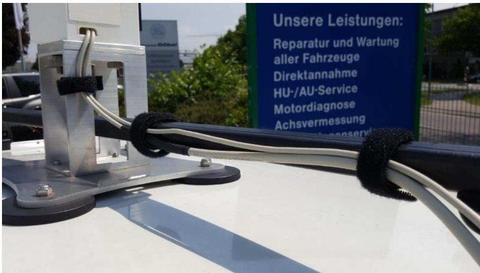
Insert the data cable and power cable through the right rear window into the car.
