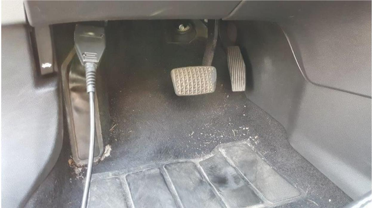
Connect the other end of the OBD2 adapter cable to the data cable. Secure it with the two thumbscrews.
