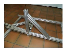
Connect to the center beam. Erect the camera pole to make sure the vertical pole and the camera pole align.
