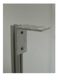
Mount the camera holder to the camera pole. In the picture the right end of the camera holder faces to the rear of the vehicle. Use 2 bolts with washer springs and 2 nut-stones. Tighten the bolts.
