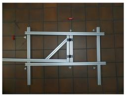
Arrange the 2 crossbeams (vertical, 80cm) and the right beam (top, 108 cm) and the center beam (bottom, 108 cm) as shown.
