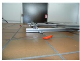
Connect the 2 crossbeams, the camerabase-profile, the right beam and the center beam with the 6 x-connectors.
