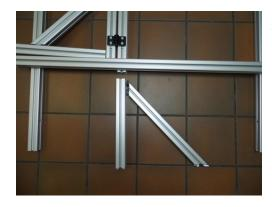
Arrange the vertical pole (36 cm) and the 45-degree profile (45 cm) as shown.
