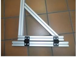
Mount the camera-base profile with 2 hinges and 8 bolts and 8 nutstones.
