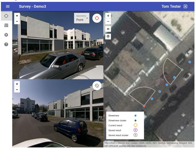
Ideally the object should be visible in the center of both top and bottom streetviews right after the map click. Photogram automatically picks two streetviews with an optimal 90 degree angle between the two stretviews.
